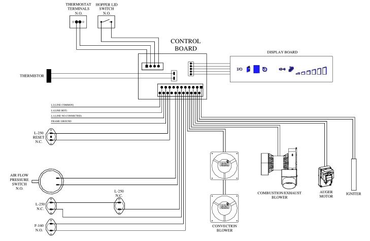
Figure 26 Electrical diagram
